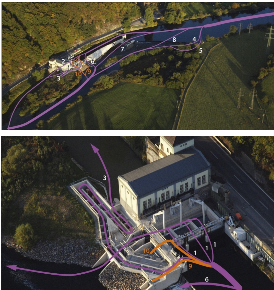
Figure 3.3. The different routes downstream migrating fish can use to pass the Unkelmühle power station: 1) via custom-made openings in the racks that leads fish to a route outside the turbines via the flushing channel, 2) through turbines if they slip through the bar spacing of the racks, 3) through the vertical slot fish passage constructed for upstream migrants, 4) through the nature-like fishway, 5) through the canoe pass, 6) via the ice gate, 7) over the spillway gate, 8) over the dam, 9) via the bottom bypass for eel, and 10) via side bypasses for eel (the two latter, indicated in orange, are only in operation during the eel run in the autumn, which was 12 August - 17 December 2014 and 24 August - 15 December 2015). Numbers in both panels refer to the different migration routes. Photos: Wikimedia Commons.
