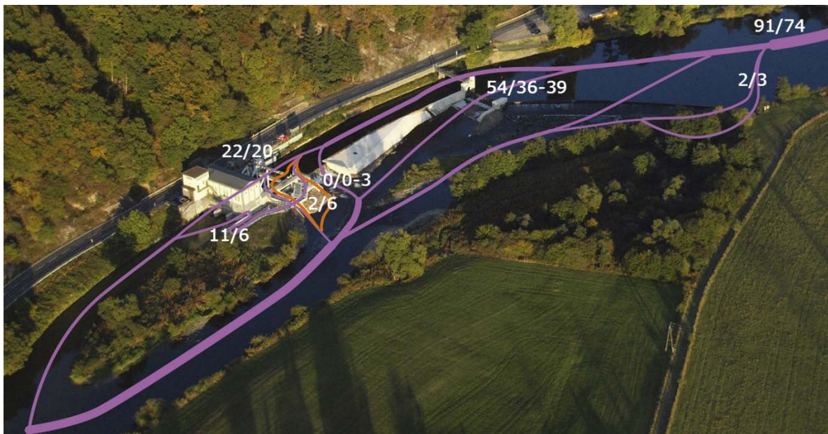
Figure 4.2. Number of eels tagged in 2014/2015 that used the different migration routes when passing the power station. Total number of eels passing along a known migration route was 91 in 2014 and 74 in 2015. Most of the eels passed over the spillway gate, or followed the migration route towards the bar racks in front of the turbines, where they were guided to a route outside the turbines via the flushing channel. Some eels used the vertical slot fish passage, the bottom bypass and the nature-like fishway or canoe pass. Three eels in 2015 passed when the ice gate was open, and for these we were not able to separate whether they migrated past the spillway gate or ice gate.
