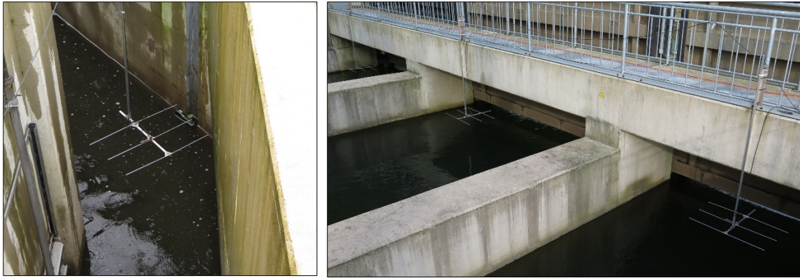
Figure 2.7. Detailed recording of the movements of tagged fish at the power stations was done by using a network of stationary receivers with antennas covering all possible migration routes. Lotek model SRX 600 data loggers were used with 3-, 4-, 6- and 9-element Yagi-antennas or co-axial antennas used underwater or in air. When a tagged fish was within the detection range of an antenna, date, time, individual fish code, signal strength from the transmitter and individual antenna number were automatically recorded and stored by the receiver and later downloaded to a computer. Photos from Unkelmühle by Stein Are Sæther and Eva B. Thorstad.
