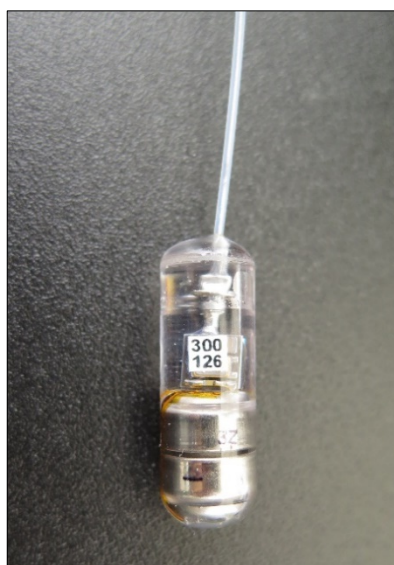
Figure 2.2. The eels were tagged with small radio transmitters (dimensions 9 x 30 mm; mass in air 4.3 g). Photos by Eva B. Thorstad.
